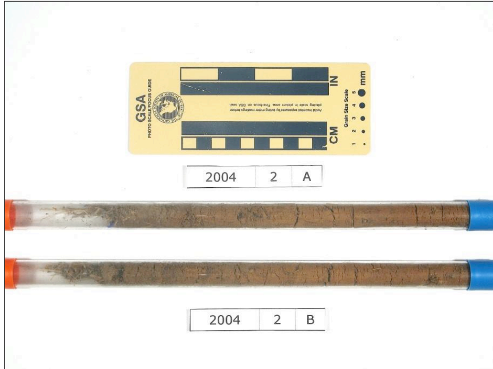
Figure 13. A Photograph of a typical soil core sample. An orange cap was used to designate the top of the soil column and a blue cap to distinguish the bottom of the core. Photograph was taken by T. Grundl, September 2007.
